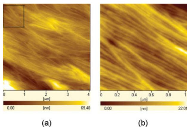
**FIGURE 4** (a) AFM height image of the concave band of the ring-banded spherulite and (b) the magnification of the boxed region in (a). [Color figure can be viewed in the online issue, which is available at [www.interscience.wiley.com](http://www.interscience.wiley.com).]
