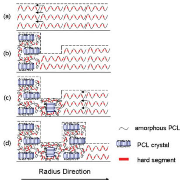
**SCHEME 2** Model of the ring-banded spherulite formation. [Color figure can be viewed in the online issue, which is available at [www.interscience.wiley.com](http://www.interscience.wiley.com).]
