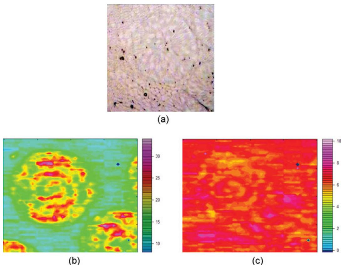
**FIGURE 6** Optical image (a) and FTIR images ( $256 \times 256 \mu\text{m}^2$ ) showing the distribution of (b) PCL soft segment based on  $A_{\nu(\text{CH}_2)}/A_{\delta(\text{NH})}$  and (c) hard segment based on  $A_{\delta(\text{NH})}/A_{\nu(\text{CH}_2)}$  with the added color scale.
