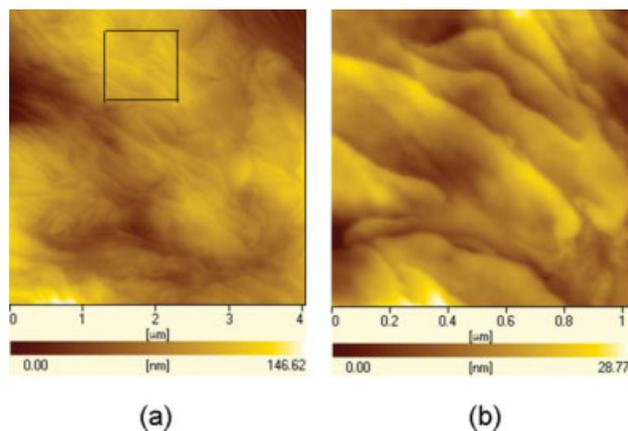
**FIGURE 3** (a) AFM height image of the convex band of the ring-banded spherulite and (b) the magnification of the boxed region in (a). [Color figure can be viewed in the online issue, which is available at [www.interscience.wiley.com](http://www.interscience.wiley.com).]
