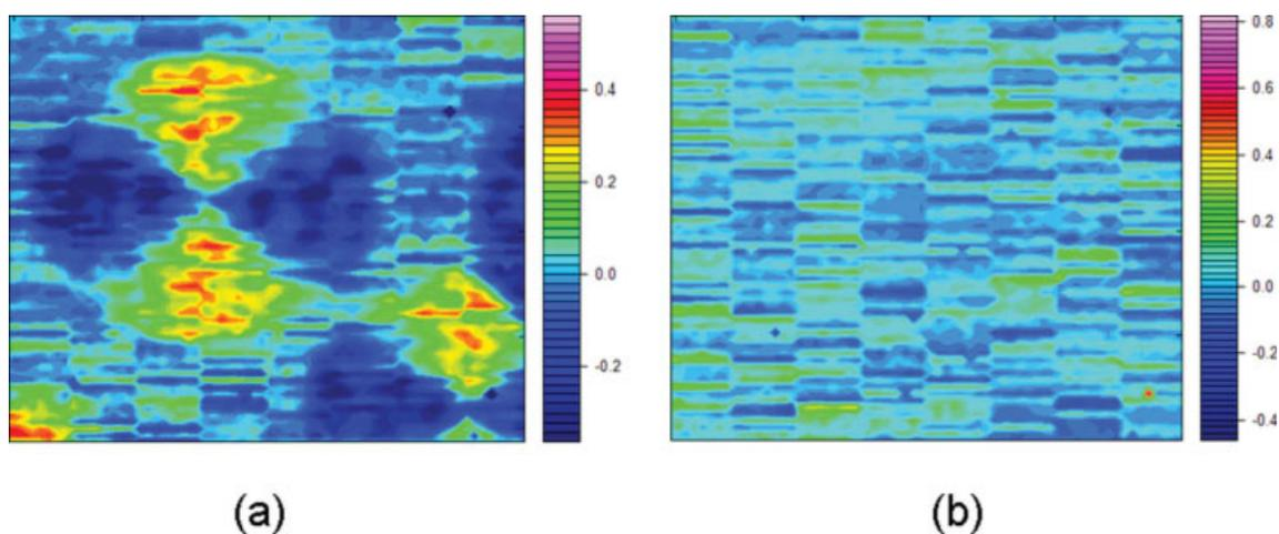
**FIGURE 5** The corresponding orientation function images ( $256 \times 256 \mu\text{m}^2$ ) of (a) PCL soft segment ( $f_{SS}$ ) and (b) hard segment ( $f_{HS}$ ) with the added color scale.
