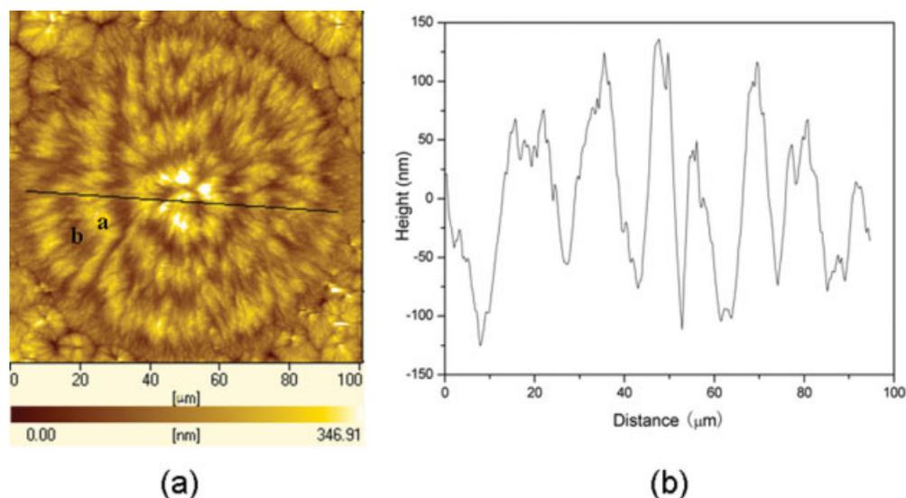
**FIGURE 2** (a) AFM height image of the ring-banded spherulite and (b) the corresponding height profile along the added black line shown in (a). [Color figure can be viewed in the online issue, which is available at [www.interscience.wiley.com](http://www.interscience.wiley.com).]
