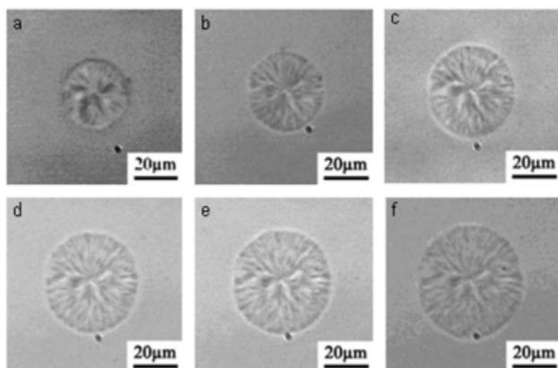
**FIGURE 7** Rhythmic growth of ring-banded spherulite at  $T_c = 46\text{ }^\circ\text{C}$  (●, convex band; ○, concave band). a–f are the optical images corresponding to the labels in the upper figure.
