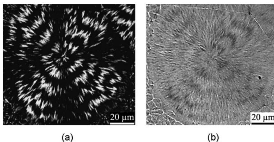
**FIGURE 1** Optical micrographs of the PEU crystallized at  $48 \text{ }^\circ\text{C}$  (a) under crossed-polarized light and (b) under unpolarized light.
