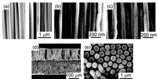
**Figure 3** SEM micrographs of PC/PS nanorods prepared by infiltrating the AAO template with a PC/PS melt: (a, d, e) 300 nm; (b) 65 nm; (c) 35 nm. (a, b, c, d) cross section of the nanorod array; (e) top view of the nanorod array with the tips of the nanorods removed.
