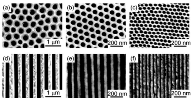
**Figure 2** SEM micrographs of AAO templates with pore diameters of (a, d) 300 nm; (b, e) 65 nm; (c, f) 35 nm. (a, b, c) top view of the AAO templates; (d, e, f) cross section of the AAO templates.
