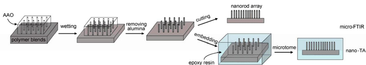
**Figure 1** Schematic of sample preparation for micro-FTIR and nano-TA measurement.
