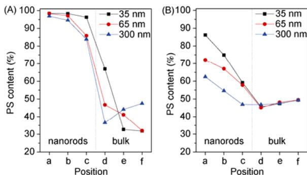
**Figure 5** PS content at different positions in nanorods/film of PC/PS blends (A) and PPO/PS blends (B).
