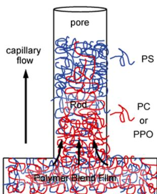
**Figure 7** Schematic illustration of the formation of gradient composition distributed polymer blends in nanopores.
