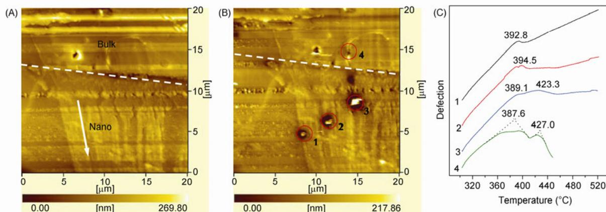
**Figure 6** AFM images of PC/PS nanorods/film with rod diameter of 300 nm before (A) and after (B) indent in the nano-TA measurement, (C) temperature dependence of the cantilever deflection in nanorods at spots 1, 2, 3, and in bulk film at spot 4.
