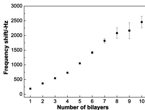
**Fig. 1** Bilayer deposition of PGM and P(AAm-AAPBA) on the (PDDA/PSS)<sub>2</sub>/PDDA-coated silver electrode monitored by QCM. The subscript denotes the number of bilayers deposited. The concentrations of PGM and P(AAm-AAPBA) were both 0.1 mg mL<sup>-1</sup> in 0.01 M PBS (pH 9.0) containing 0.5 M NaCl.
