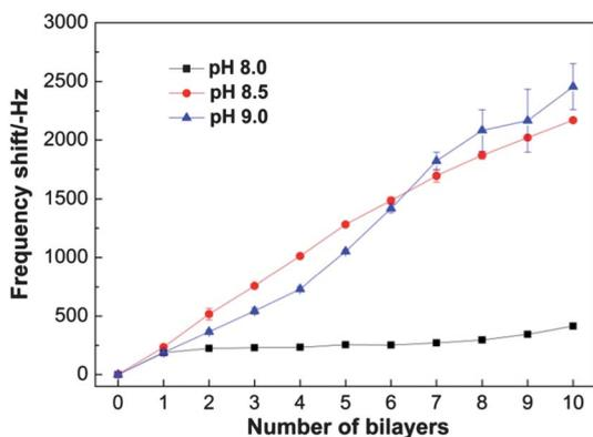
**Fig. 4** Frequency shift of PGM/P(AAm-AAPBA) multilayer film under different pH values. The concentrations of PGM and P(AAm-AAPBA) were both 0.1 mg mL<sup>-1</sup> in 0.01 M PBS containing 0.5 M NaCl.
