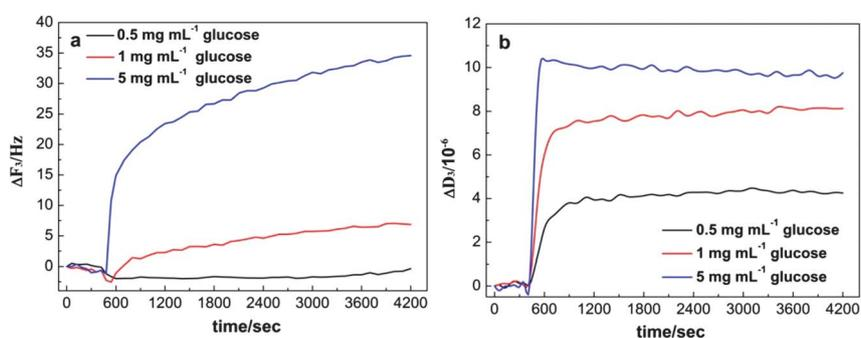
**Fig. 6** QCM-D data for the disintegration of PGM/P(AAm-AAPBA) films in various concentrations of glucose at pH 9.0. (a) The corresponding frequency shift *vs.* time for the third overtone. (b) The corresponding dissipation shift *vs.* time for the third overtone.
