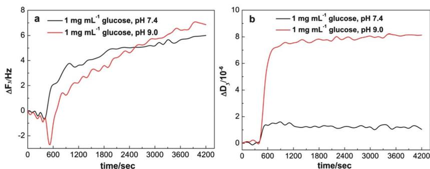
**Fig. 7** QCM-D data for the disintegration of PGM/P(AAm-AAPBA) films at pH 7.4 and 9.0. (a) The corresponding frequency shift vs. time for the third overtone. (b) The corresponding dissipation shift vs. time for the third overtone.
