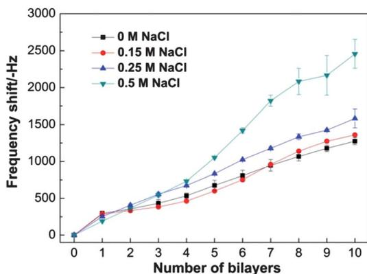
**Fig. 3** Frequency shift of PGM/P(AAm-AAPBA) multilayer film dependent on the concentration of NaCl. The concentrations of PGM and P(AAm-AAPBA) were both 0.1 mg mL<sup>-1</sup> in 0.01 M PBS (pH 9.0).
