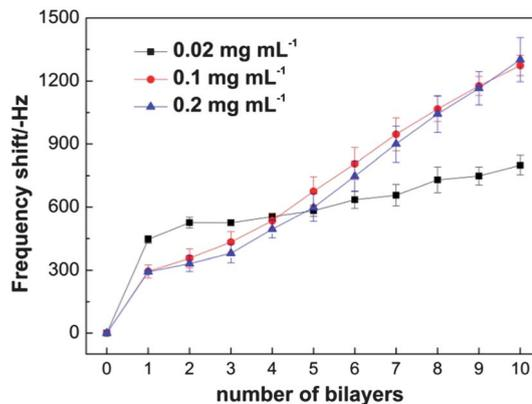
**Fig. 5** Frequency shift of PGM/P(AAm-AAPBA) multilayer film dependent on PGM concentration. The concentration of P(AAm-AAPBA) was 0.1 mg mL<sup>-1</sup> in 0.01 M PBS (pH 9.0).
