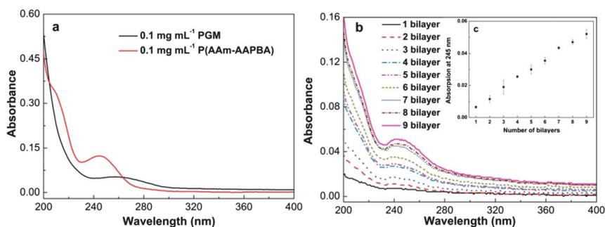
**Fig. 2** (a) Absorption spectra for PGM (0.1 mg mL<sup>-1</sup>, pH 9.0) and P(AAm-AAPBA) (0.1 mg mL<sup>-1</sup>, pH 9.0) in aqueous solution. (b) Absorption spectra for PGM/P(AAm-AAPBA) films on a silver electrode with different bilayer numbers. (c) The inset shows the step growth of the absorbance at 245 nm as a function of number of bilayers deposited. The films were fabricated in 0.01 M PBS (pH 9.0) containing 0.5 M NaCl.
