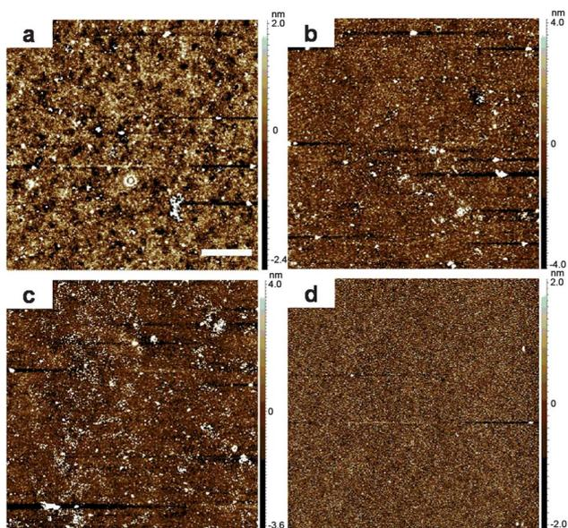
**Fig. 8** AFM height images of PGM/P(AAm-AAPBA) multilayer films immersed at two different pH values of the glucose solution. (a) 6-bilayer film without glucose, (b) 6-bilayer film immersed in PBS buffer (pH 9.0) with  $1 \text{ mg mL}^{-1}$  glucose, (c) 6-bilayer film immersed in PBS buffer (pH 7.4) with  $1 \text{ mg mL}^{-1}$  glucose and (d) the (PDDA/PSS)<sub>2</sub>/PDDA film. The image dimensions are  $10 \times 10 \mu\text{m}^2$  and the scale bar is  $20 \mu\text{m}$ .
